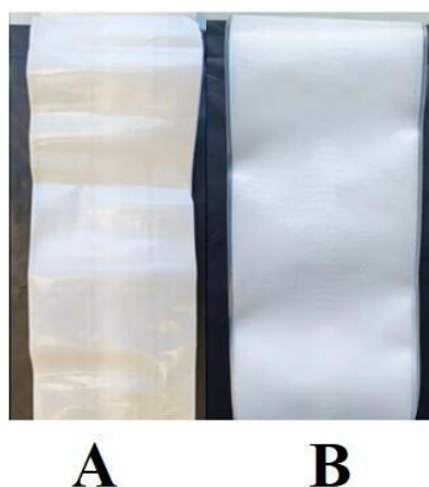
Figure 2. The external appearance of the obtained films: A) LDPE film with \text{TiO}_2 3% without ultrasound treatment, B) LDPE film with \text{TiO}_2 3% with ultrasound treatment.
