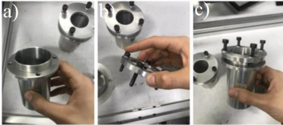
Figure 1. Apparatus for pervaporation test: a) Cup of fuel; b) Ring for sample fixation; c) System after ring fixation.
