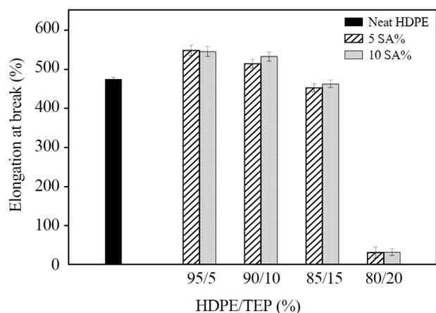
**Figure 6.** Variation of elongation-at-break for HDPE/TEP composites.
