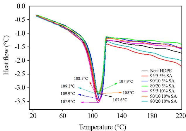
**Figure 8.** DSC thermograms of HDPE/TEP composites from the first cooling cycle showing the crystallization temperatures.
