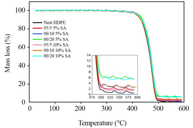
**Figure 9.** Mass loss as a function of temperature for HDPE/TEP composites.
