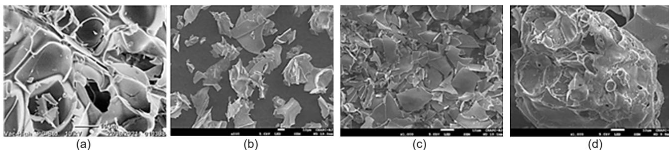
**Figure 1.** SEM images of (a) raw expanded perlite, (b) perlite after HCl treatment, (c) perlite treated with 5% SA, and (d) perlite treated with 10% SA (d).
