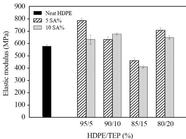
**Figure 4.** Effect of treated perlite on the elastic modulus for HDPE/TEP composites.
