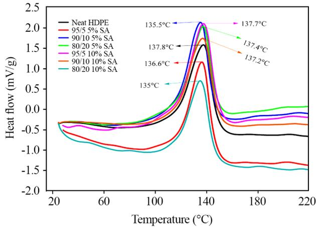
**Figure 7.** DSC thermograms of HDPE/TEP composites from the second heating cycle showing melting temperatures.
