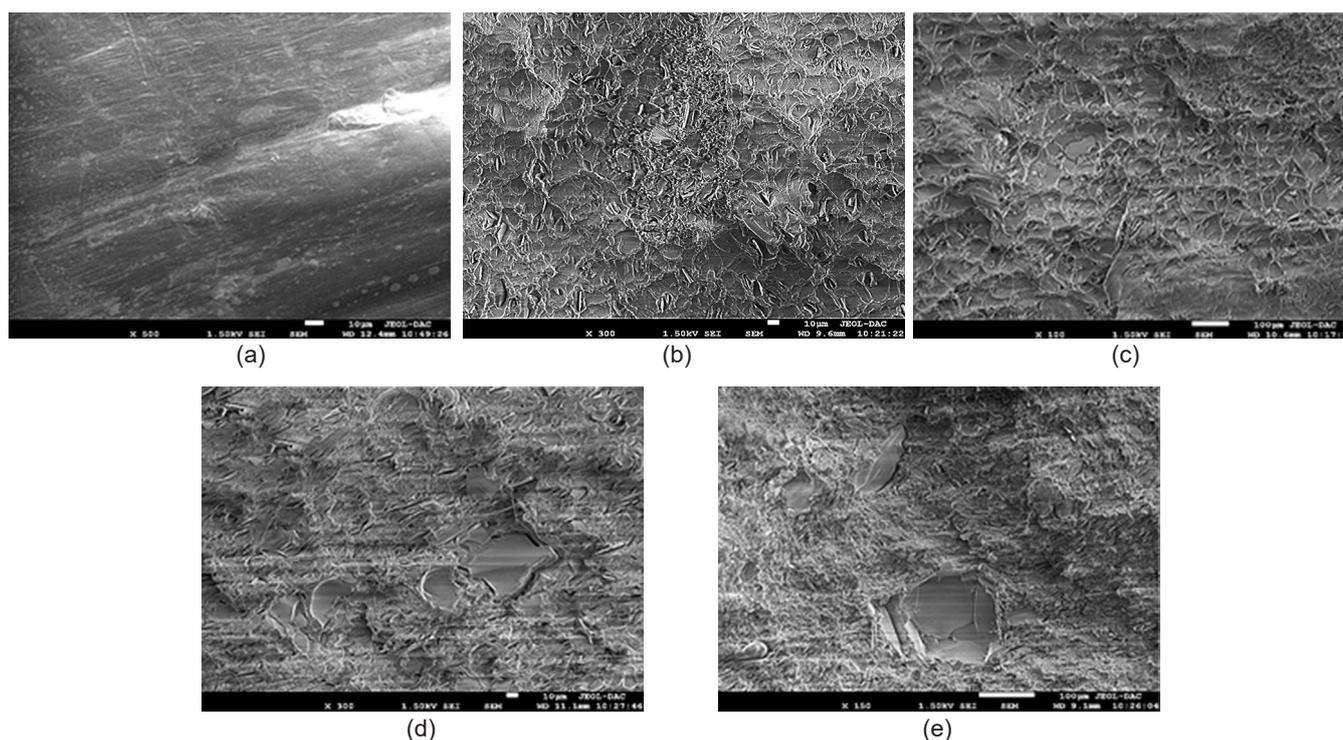
**Figure 2.** SEM images of impact-fractured surfaces of (a) neat HDPE, (b) HDPE/5%TEP with 5% SA, (c) HDPE/20%TEP with 5% SA, (d) HDPE/5%TEP with 10% SA, and (e) HDPE/20%TEP with 10% SA.
