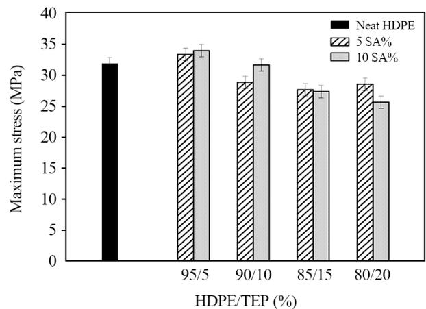
**Figure 5.** Effect of treated perlite on the maximum stress for HDPE/TEP composites.
