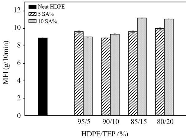
**Figure 3.** Melt flow index of HDPE/TEP composites based on perlite content and stearic acid treatment.
