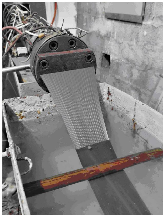
**Figure 3.** Fall of the tape into the water tank.
