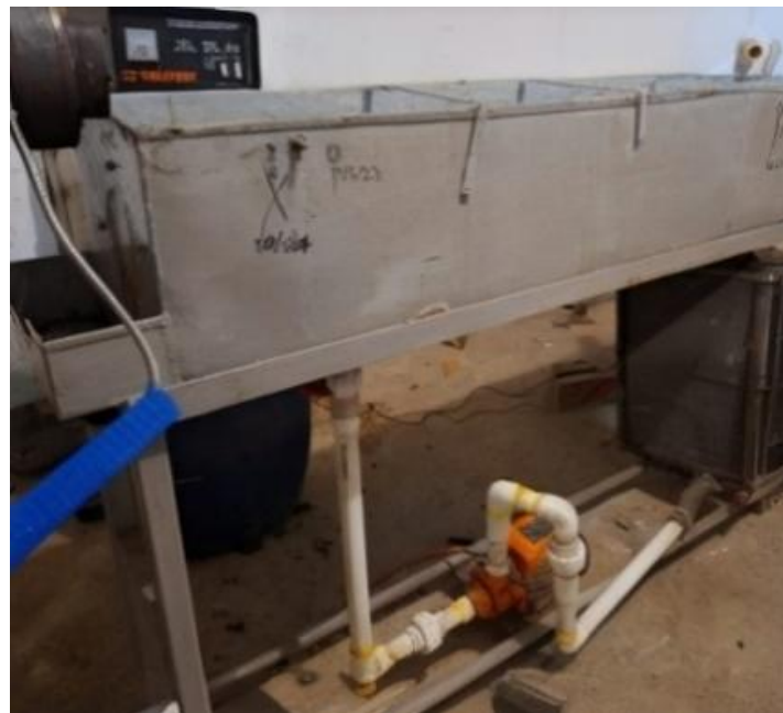
Figure 1. Cooling water tank.
