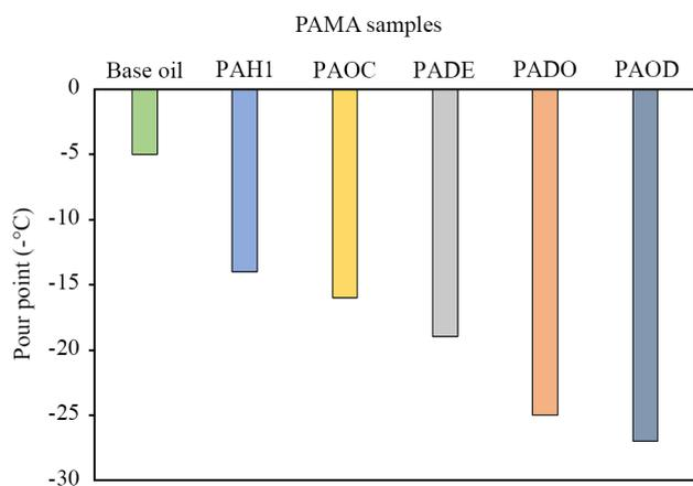
**Figure 5.** Effect of side chain length on pour point temperature of different PAMAs.
