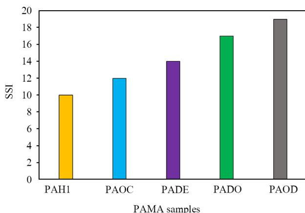
**Figure 3.** Effect of side chain length on shear stability index of different PAMAs.
