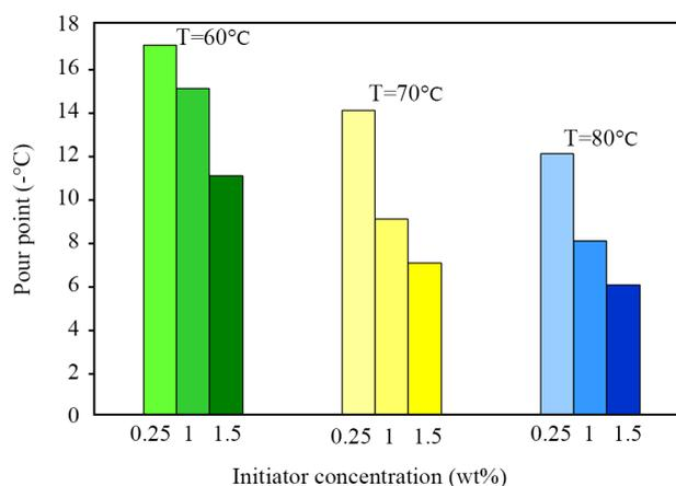
**Figure 6.** Effect of initiator concentration and reaction temperature on pour point temperature of poly(hexyl methacrylate).
