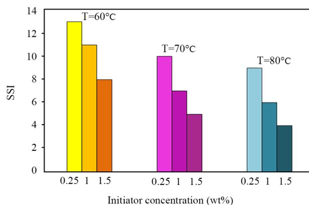
**Figure 4.** Effect of initiator concentration and reaction temperature on shear stability index of poly(hexyl methacrylate).
