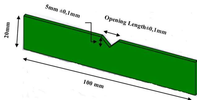
**Figure 3.** Dimensions used for HIPS and HDPE V-notched specimens.
