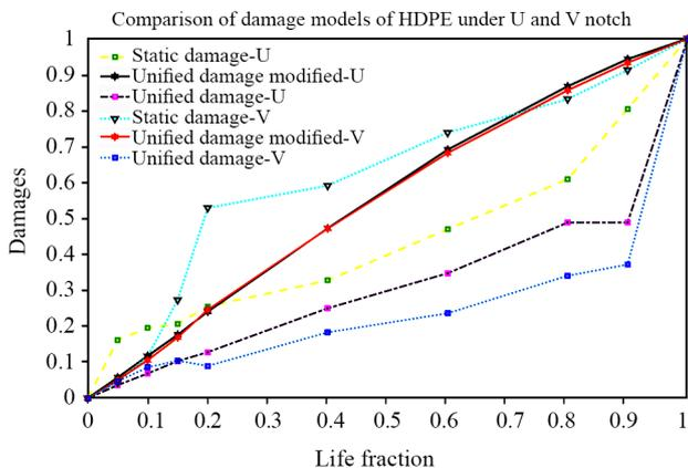
**Figure 9.** Comparison of damage in the U and V-notched HDPE.
