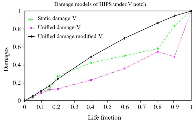
**Figure 10.** Three damage models calculated for V-notched HIPS.
