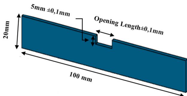
**Figure 2.** Dimensions used for HIPS and HDPE U-notched specimens.
