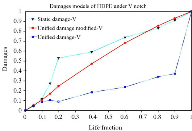
**Figure 8.** Damage patterns of V-notched HDPE.
