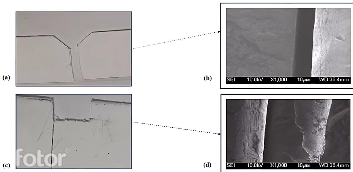
**Figures 16.** Image results for HIPS: (a) HIPS with V-notch, (b) V-notch SEM, (c) HIPS with U-notch, (d) U-notch SEM.
