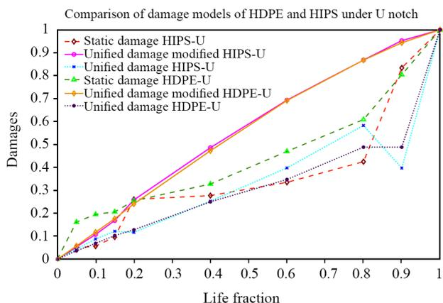
**Figure 13.** Damage comparisons of HIPS and U-notched HDPE.
