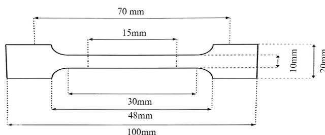
**Figure 1.** Dimensions of the HDPE and HIPS specimens used for the characterization.
