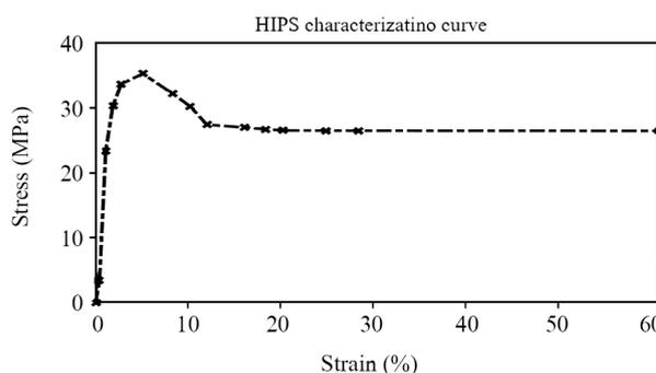
**Figure 5.** HIPS characterization curve.
