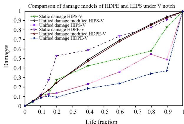
**Figure 14.** Damage comparisons of HIPS and V-notched HDPE.
