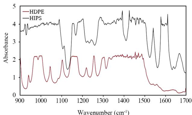
**Figure 4.** HDPE and HIPS IR spectrometry.
