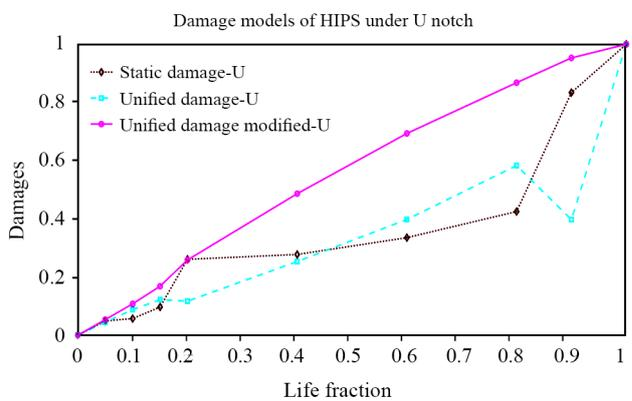
**Figure 11.** Three damage models calculated for U-notched HIPS.
