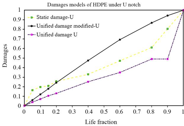
**Figure 7.** Damage patterns of U-notched HDPE.
