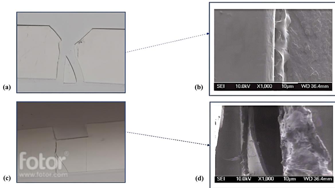
**Figure 15.** Image results for HDPE: (a): HDPE with V-notch, (b): V-notch SEM, (c): HDPE with U-notch, (d): U-notch SEM.
