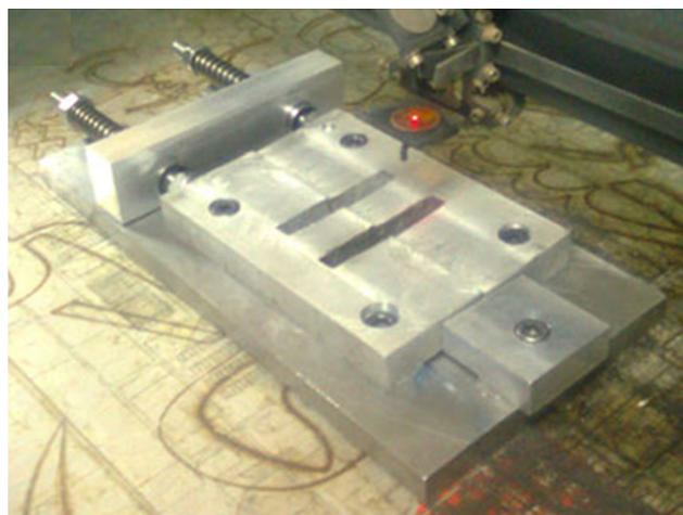
**Figure 3.** Fixture for making pressure during welding operation.
