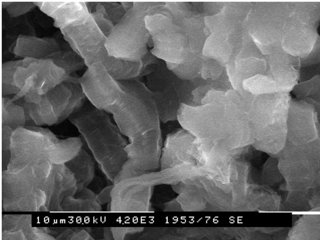
**Figure 1.** SEM image of nanocomposite nascent particles with 2.5 vol% of GnP.
