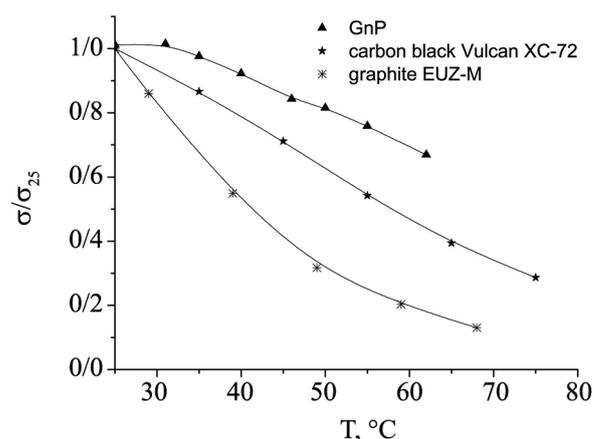
**Figure 6.** Relative temperature dependencies of conductivity for composites based on different carbon fillers with a conductivity  $\sigma_{dc\perp} \sim 10^{-4}$  S/m.
