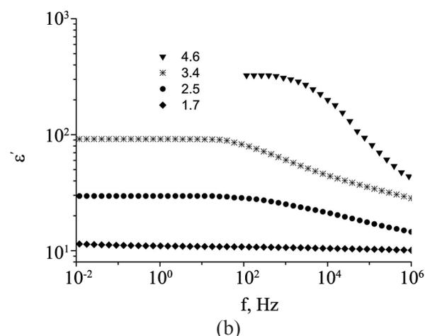
**Figure 3.** Frequency dependencies of conductivity (a) and dielectric permittivity (b) for UHMWPE/GnP composites with different filler concentrations (vol%).
