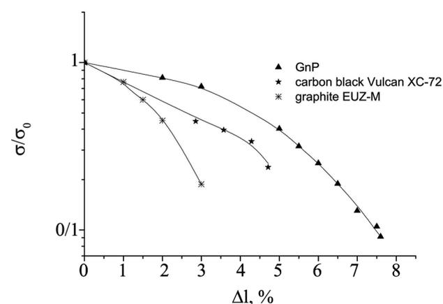
**Figure 7.** Relative deformation dependencies of conductivity for composites based on different carbon fillers with a conductivity  $\sigma_{dc\perp} \sim 10^{-4}$  S/m.
