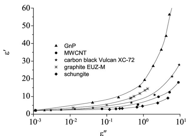
**Figure 5.** Dependency of dielectric permittivity versus dielectric loss for composites based on different carbon fillers.
