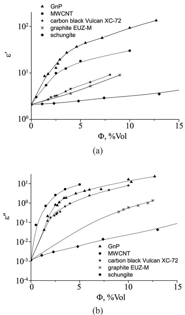
**Figure 4.** Concentration dependencies of dielectric permittivity  $\varepsilon'$  (a) and loss  $\varepsilon''$  (b) at frequency 11GHz for composites based on different carbon fillers.
