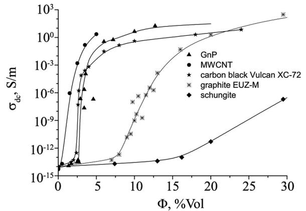
**Figure 2.** Concentration dependencies of  $\sigma_{dc}$  for composites based on different carbon fillers.
