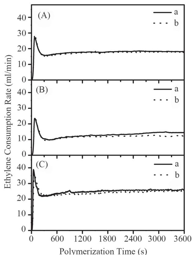
**Figure 8.** Kinetic curves of ethylene homopolymerization with/without hydrogen. (A): i-Mg/Ti/Si, Al/Ti=5, (a) without H<sub>2</sub>, (b) with H<sub>2</sub>, corresponding to Run 2, 6; (B): i-V/Ti/Si, Al/Ti=2.5, (a) without H<sub>2</sub>, (b) with H<sub>2</sub>, corresponding to Run 10, 15; (C): i-Mg/V/Ti/Si, Al/Ti=10, (a) without H<sub>2</sub>, (b) with H<sub>2</sub>, corresponding to Run 21, 24. Conditions: catalyst 100 mg, ethylene 0.15 MPa, n-heptane 70 mL, TIBA, 1 h, H<sub>2</sub> 10 mL.
