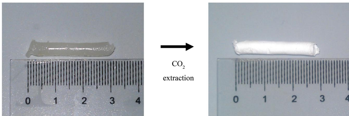
**Figure 1.** Photographs of a piece of PE gel prepared in decalin at  $C_{\text{pol}} = 10 \text{ wt}\%$ , before and after complete solvent extraction via supercritical carbon dioxide (units of the ruler are cm).
