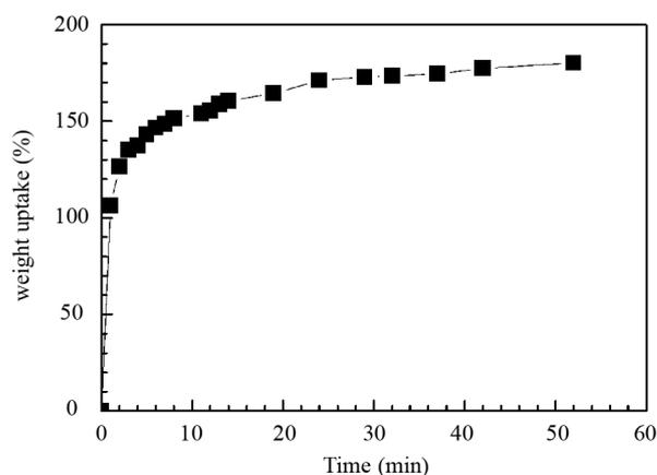
**Figure 5.** Sorption kinetics at room temperature of white mineral oil in a PE aerogel with a porosity of 90%.
