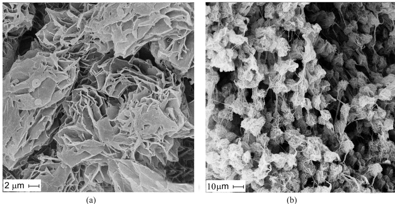
**Figure 2.** SEM images of a polyethylene aerogel with porosity  $P = 90\%$  obtained from a gel prepared in decalin with  $C_{\text{pol}} = 10$  wt %, after complete solvent extraction by  $\text{SC-CO}_2$ .
