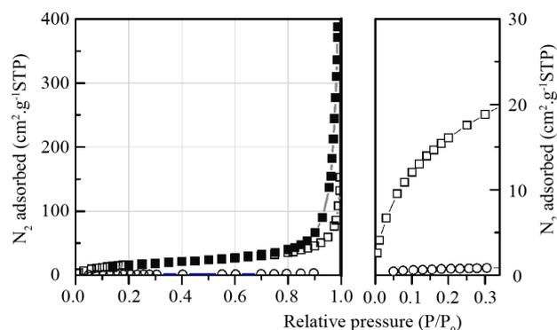
**Figure 4.** Left: volumetric  $\text{N}_2$  adsorption-desorption isotherms at 77 K in the 0-0.99  $P/P_0$  range of a PE aerogel ( $\blacksquare, \square$ ) and PE commercial powder ( $\circ$ ). For the aerogel, the empty and filled scatters refer to the adsorption and desorption branches, respectively. Right: volumetric  $\text{N}_2$  adsorption isotherms in the 0-0.3  $P/P_0$  range of a PE aerogel ( $\square$ ) and PE commercial powder ( $\circ$ ).
