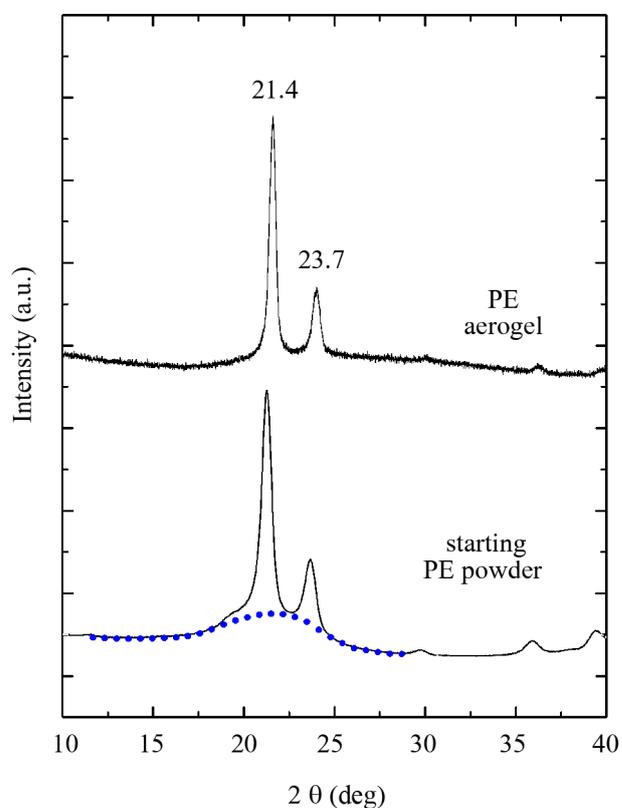
**Figure 3.** X-ray diffraction of commercial starting PE powder and PE aerogel.
